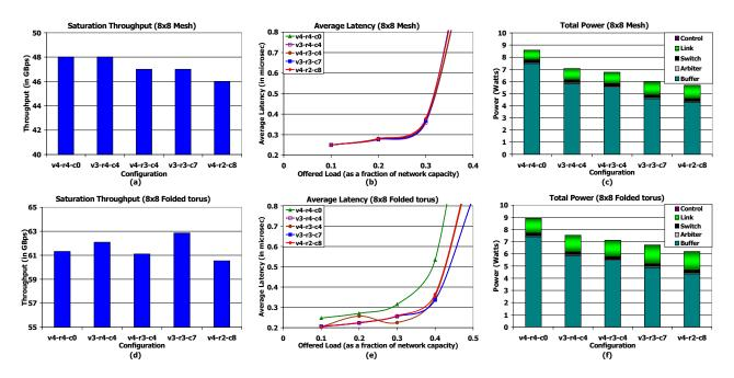
Figure 8: Saturation Throughput, Average Latency and Overall network power (at network load = 0.5) under Uniform Traffic for  $8 \times 8$  mesh and folded torus networks.
