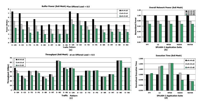
Figure 10: (a) Buffer power for synthetic traffic (b) Normalized Overall network power for SPLASH-2 benchmarks (c) Throughput for synthetic traffic (d) Normalized Execution time for SPLASH-2 benchmarks. Synthetic traffic patterns (Uniform (UN), Complement (CO), Tornado (TO), Perfect Shuffle (PS), Bit-Reversal (BR), Matrix Transpose (MT), Neighbor (NE) and Butterfly (BU)) are considered under both static (S) and dynamic (D) buffer allocation schemes.
