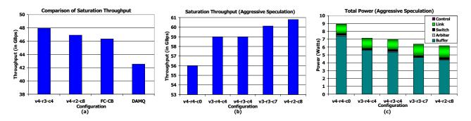
Figure 9: (a) Throughput Comparison for the 4-3-4 and 4-2-8 iDEAL configurations, Fully Connected Circular Buffers (FC-CB) and Dynamically Allocated Multiqueue (DAMQ) Buffers, under Uniform traffic for  $8 \times 8$  mesh network. (b) Throughput and (c) Overall network power (at network load = 0.5) for Aggressive Speculation using 8 credits, under Uniform traffic for  $8 \times 8$  folded torus network.
