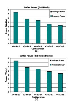
Figure 7: Buffer power for  $8 \times 8$  mesh and folded torus networks under Uniform traffic, at network load = 0.5. In the notation  $vn_V - rn_R - cn_C$ ,  $n_V$  is the number of VCs per input port,  $n_R$  is the number of router buffers per VC and  $n_C$  is the number of link buffers.
