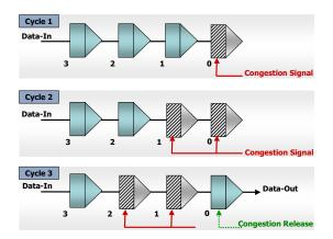
Figure 4: Data-flow control in the repeater stages during congestion.
