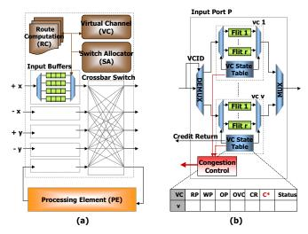
Figure 5: (a) A generic  $5 \times 5$  NoC router architecture (b) The proposed static buffer allocation with congestion control.
