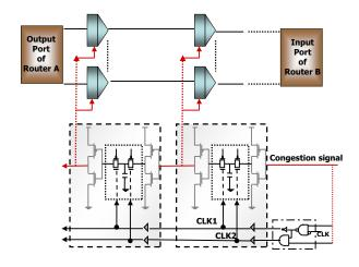
Figure 2: Proposed switched-capacitor based control block.
