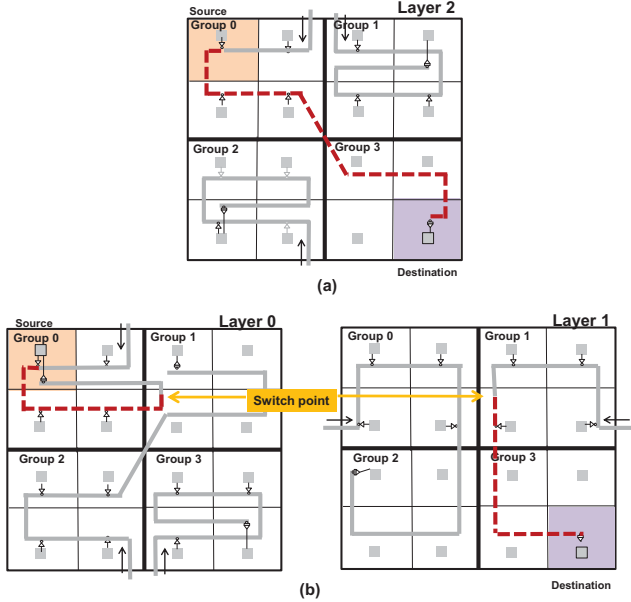
Figure 3: (a) Static communication between the source in Group 0 and destination in Group 3. (b) Illustration of reconfiguration between Groups 0 and 3 using partial waveguides from layers 0 and 1.
